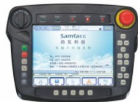
三轴伺服驱动标配为触摸式操控器 Three-axis servo drive is standard as a touch controller
